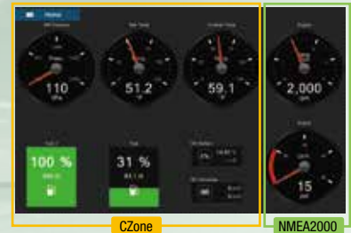
CZone, engine, navigation and various NMEA2000 data can be laid out on the same screen.
